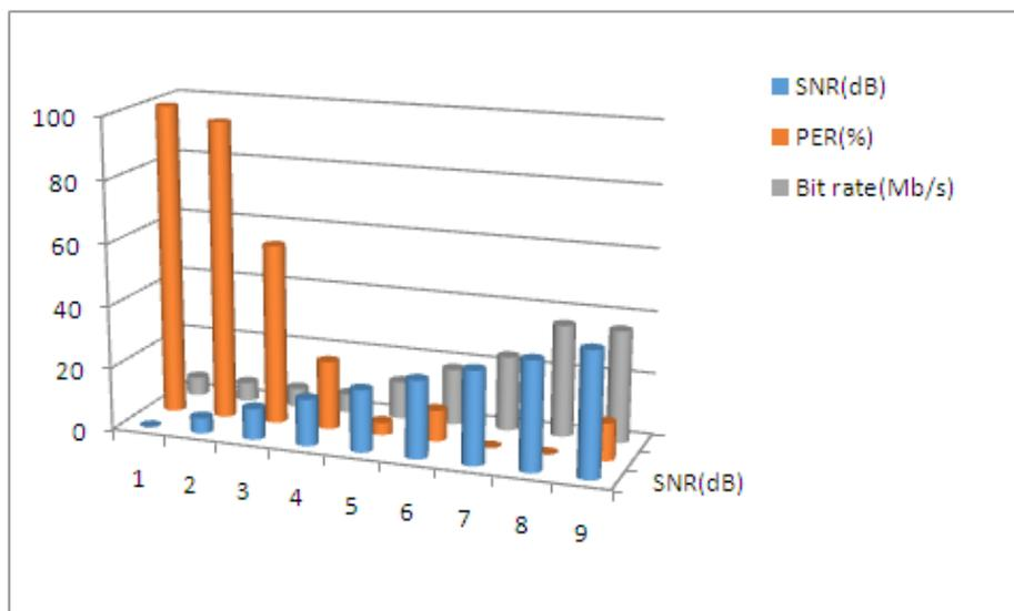
**Figure 11:** SNR (dB) Vs PER (%) and Bit rate (Mb/s) when max Doppler shift is 100 Hz.
