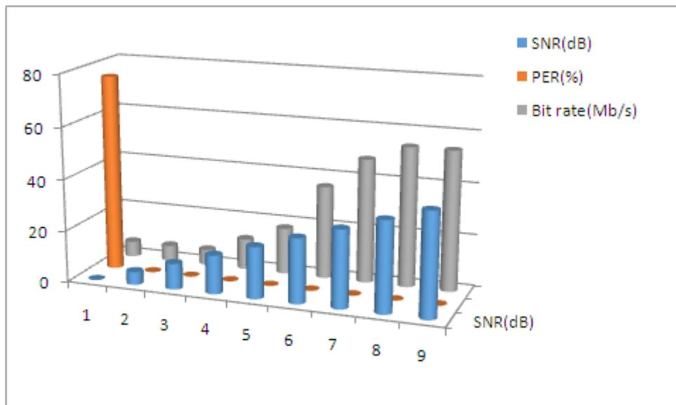
Figure 4: SNR (dB) Vs PER (%) and Bit rate (Mb/s) when max Doppler shift is 200 Hz.
