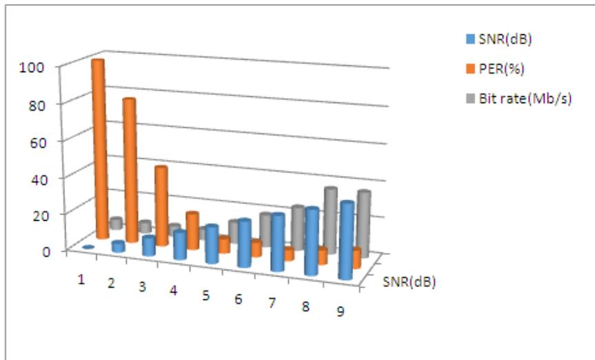
**Figure 10:** SNR (dB) Vs PER (%) and Bit rate (Mb/s) when max Doppler shift is 200 Hz.
