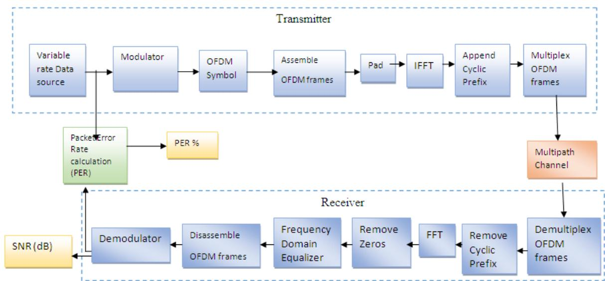
Figure 3: 802.11a WLAN Physical Layer Model
