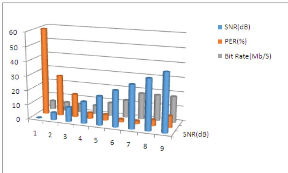
**Figure 7:** SNR (dB) Vs PER (%) and Bit rate (Mb/s) when max Doppler shift is 200 Hz.
