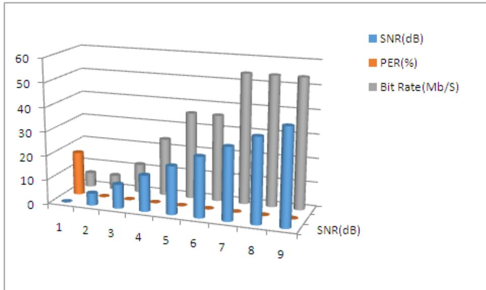
Figure 8: SNR (dB) Vs PER (%) and Bit rate (Mb/s) when max Doppler shift is 100 Hz.
