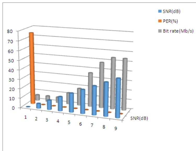
Figure 6: SNR (dB) Vs PER (%) and Bit rate (Mb/s) when max Doppler shift is 300 Hz.
