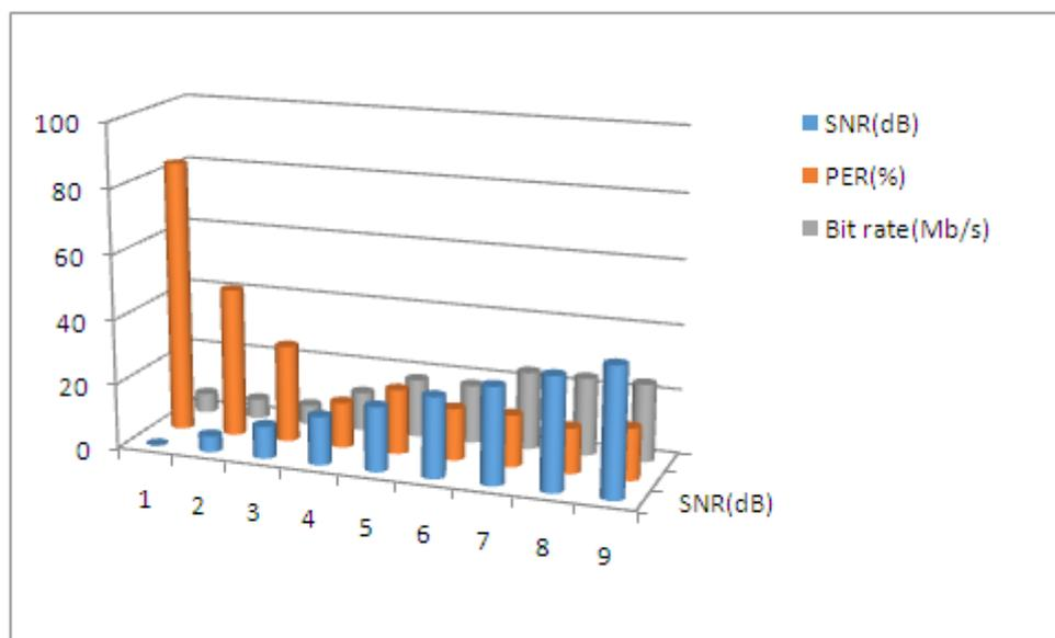
**Figure 12:** SNR (dB) Vs PER (%) and Bit rate (Mb/s) when max Doppler shift is 300 Hz.
